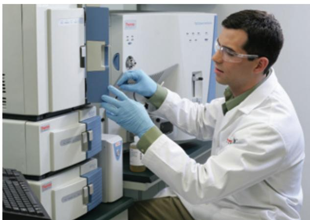
2.4  $\mu\text{m}$  Hypersil BDS columns can also be used with modern ultra high pressure liquid chromatography (UHPLC) instruments, including the Thermo Scientific Accela High Speed LC.
