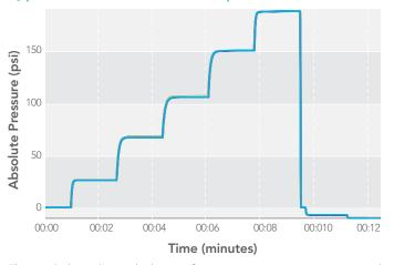
This graph shows the overlaid output from ten pressure sensors monitoring the same fluidic channel. High reproducibility and the capability for simultaneous reading of multiple sensors make the units extremely valuable for instrumentation applications. In this plot, the sensors are responding to a series of pressure increases over the sensor range.
